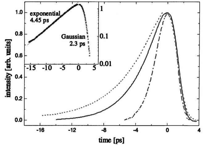
FIG. 3. FEL pulse shape as measured at three different settings of the cavity detuning,  $-7.65$  (dotted line),  $-4.9$  (solid line), and  $-1.65\ \mu\text{m}$  (dash-dotted line). The inset shows the pulse generated at  $-7.65\ \mu\text{m}$  in a semilogarithmic format together with a fit to an exponential on the rising edge.
