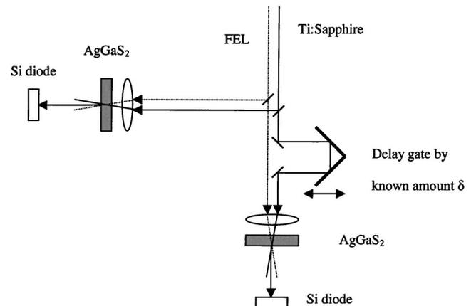
FIG. 1. Schematic of the experimental setup for differential optical gating [7] at a wavelength of  $6.3 \mu\text{m}$ . The Ti:sapphire (gate) beam is split into two arms, one of which is delayed with respect to the other by a known amount  $\delta$ . In both arms the FEL beam and the gate beam copropagate through a AgGaS<sub>2</sub> crystal and the corresponding sum-frequency signals are detected by silicon diodes.
