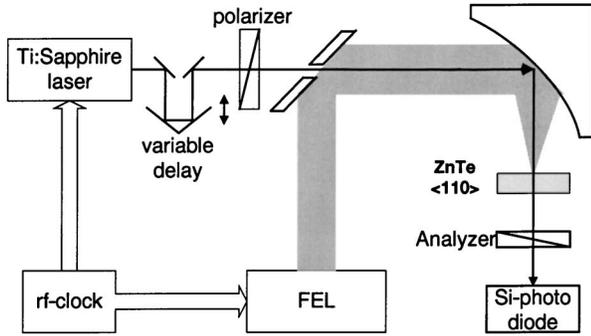
FIG. 2. Schematic of the electro-optic cross-correlation setup. The FEL-induced birefringence in a ZnTe crystal is probed with a synchronized Ti:sapphire laser. A Si photodiode measures the Ti:sapphire intensity passing through a pair of crossed polarizers.
