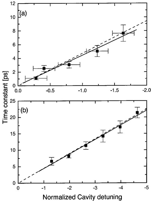
FIG. 4. Measured and simulated exponential time constants of the rising edge of the pulse as function of cavity desynchronization. The data at  $6.3 \mu\text{m}$  from Stanford are shown in (a), while the  $150 \mu\text{m}$  wavelength data taken at FELIX are shown in (b). The solid lines are linear fits to these data; the dashed lines show the results from simulations with a 1D code [8]. See text for details.
