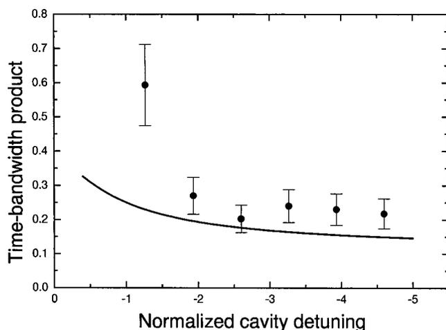
FIG. 7. Time-bandwidth product (FWHM) measured for different cavity detunings (solid dots). The product is in the range 0.2–0.3 if the optical pulse has an exponential leading edge. The product grows to 0.6 for pulses with a more Gaussian pulse shape. The solid line shows the *calculated* time-bandwidth product for pulses with an exponential leading edge and Gaussian trailing edge. See text for details.
