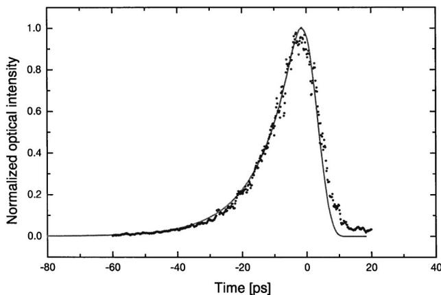
FIG. 5. A comparison of the experimental and simulated optical pulse shapes for FELIX operating at a wavelength of  $150 \mu\text{m}$  and a cavity detuning of  $-390 \mu\text{m}$ .
