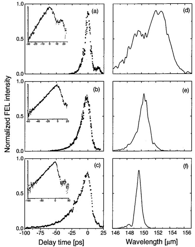
FIG. 6. Measured optical pulse shape (a)–(c) using the electro-optic cross-correlation technique described in the text, and corresponding power spectrum (d)–(f) at a wavelength of  $150 \mu\text{m}$  for different cavity detunings  $\Delta L$  of (a)  $-190$ , (b)  $-390$ , and (c)  $-690 \mu\text{m}$ . The pulse length is changed from  $8.5$  (a) to  $21$  ps FWHM in (c). The solid lines indicate exponential fits to the leading edges.
